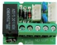
GEM-600 12/24VDC: Auto Voltage Selector Locked/Unlocked status reed switch output
